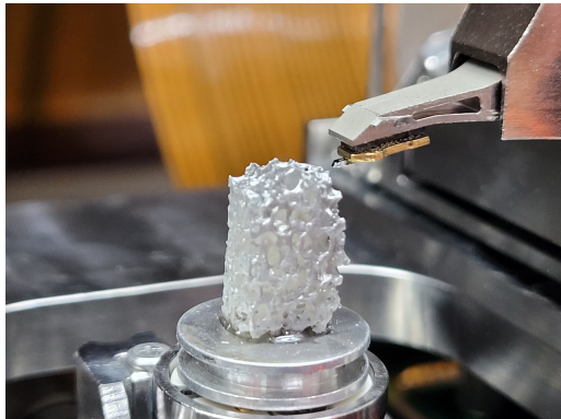
Figure 1: Bone sample mounted inside the FusionScope trunnion stage with the AFM cantilever positioned on top of the sample.
